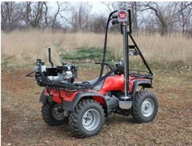
Soil sampler - ATV mounted 3-ft sampling depth
